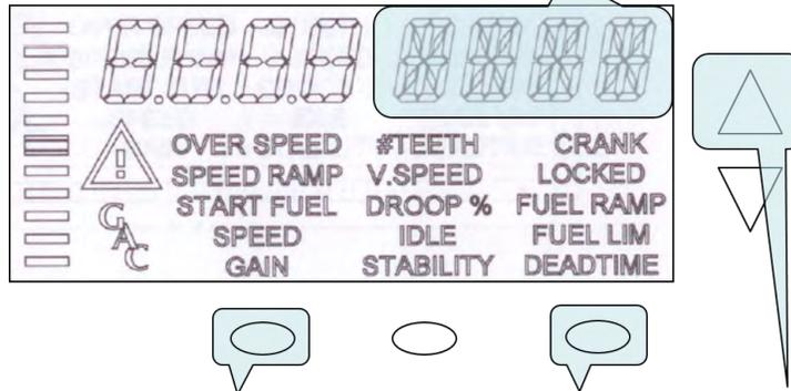
During Power Up, Press LEFT, RIGHT, and UP Buttons simultaneously and hold until "FACT" displayed. If software revision displayed, all required buttons were not pressed properly or in time.
