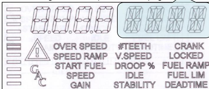
During Power Up, Press LEFT, RIGHT, and DOWN Buttons simultaneously and hold until "OEM" or "FAIL" displayed. If software revision displayed, all required buttons were not pressed properly or in time.
