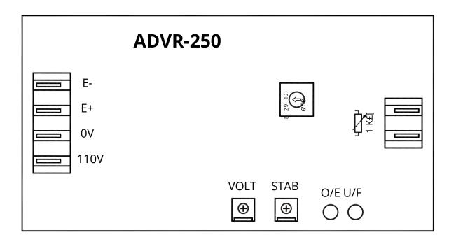
**OV 110V**: Power Supply and Sensing Input
